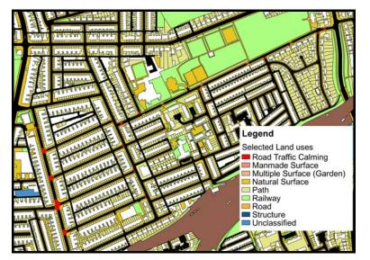
Figure 3: Areas of existing traffic calming measures (red) identified for potential SUDS retrofit
